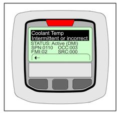
Figure 3-9. Engine Diagnostic Screen
