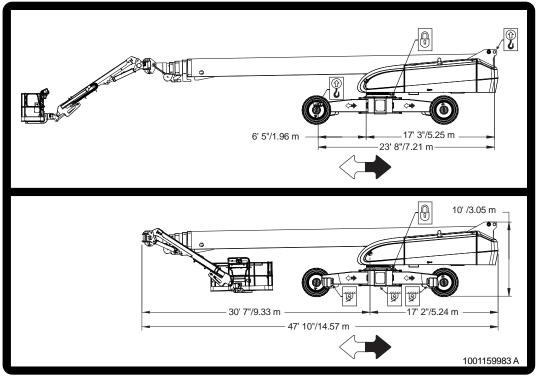
Figure 4-7. Lifting and Tie Down Chart
