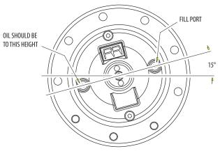
Lube Point(s) - Level/Fill Plug Capacity - 2.6 quarts (2.5 liters)  $\pm$  10% Interval - Check level every 3 months or 150 hrs of operation; change every 2 years or 1200 hours of operation
