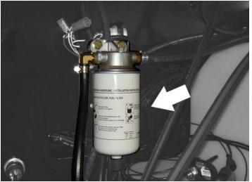
Lube Point(s) - Replaceable Element Interval - Every year or 500 hours of operation
