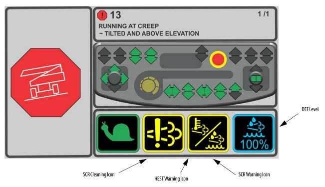
Figure 5-28. SCR Cleaning Screen - Sheet 2 of 2
