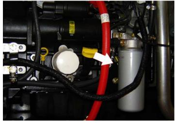
Lube Point(s) - Replaceable Element Interval - Every year or 500 hours of operation
