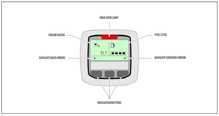
Figure 3-10. Ground Control Console Display Gauge
