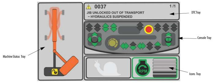
Figure 5-6. Machine Operating Screen
