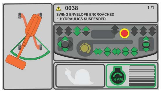
Figure 5-17. Swing DTC Screen
