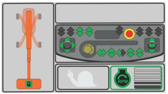
Figure 5-19. Jib Locked Screen
