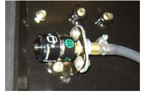
Lube Point(s) - Replaceable Element Interval - Every 6 months or 300 hours of operation or as indicated by the condition indicator Comments - Check dust valve for dirt daily
