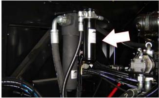
Lube Point(s) - Replaceable Element Interval - Change after first 50 hours and every 6 months or 300 hours thereafter. 7. High Pressure Filter
