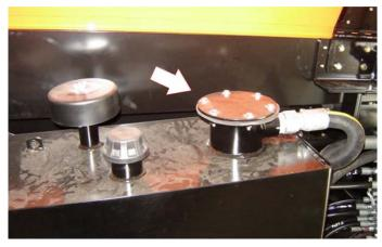
Lube Point(s) - Replaceable Element Interval - Change after first 50 hours and every 6 months or 300 hours thereafter. 5. Hydraulic Tank Breather
