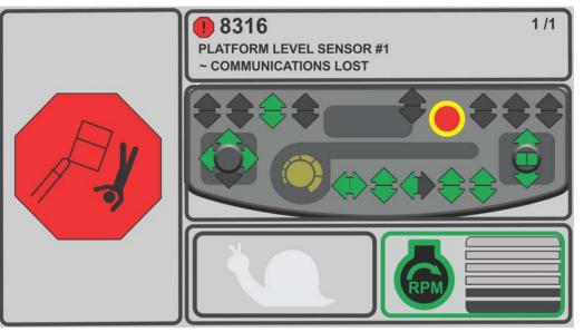
Figure 5-14. Level System DTC Screen
