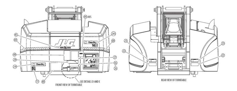
Figure 4-10. Decal Location Sheet 3 of 9
