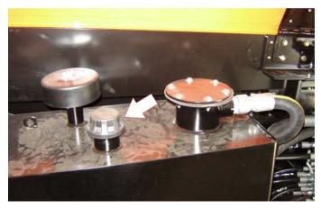
Lube Point(s) - Fill Cap Capacity - 75 Gallons (208 liters) Tank to Full Mark 82 Gallons (310.4 L) System Lube - HO Interval - Check level daily. Change every 2 years or 1200 hours of operation.
