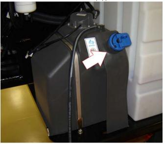
Lube Point - Fill Cap Lube - DEF Capacity - 5.7 gal. (21.5 L)
