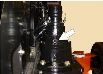
Lube Point(s) - Fill Plug Capacity - 3 qt. (2.8 L) Lube - GL-5 Interval - Check level every 150 hrs/Change every 1200 hours of operation. Fill to cover ring gear. 3. Wheel Drive Hub
