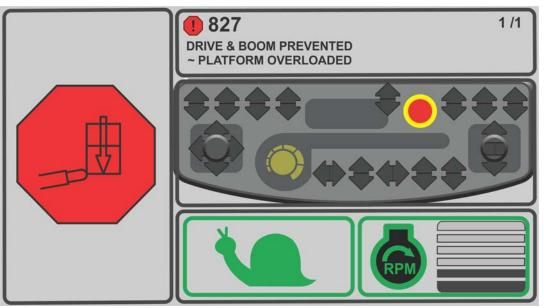
Figure 5-15. Overload DTC Screen
