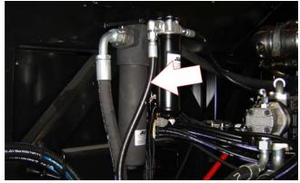
Lube Point(s) - Replaceable Element Interval - Change after first 50 hours and every 6 months or 300 hours thereafter.
