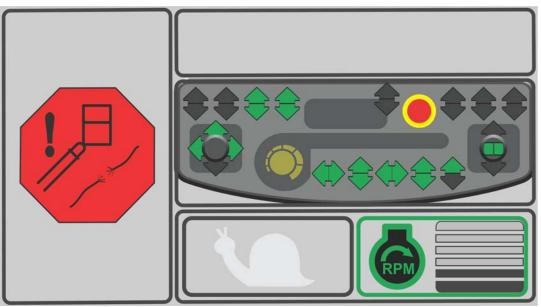
Figure 5-13. Broken Cable Screen
