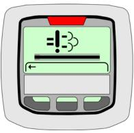
5. After the cleaning process is complete, the engine will run for approximately 5 minutes to allow the Engine and Exhaust After Treatment (EAT) to cool down. The Indicator Gauge will display the "Regen Complete" screen as shown and the HEST indicator will no longer be illuminated.
